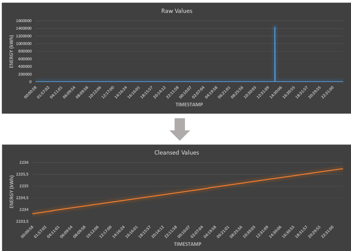
Figure 25. Hampel Filter applied on an energy consumption data set
