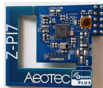
Figure 19. (left) 32 GB Micro SD, (right) Z-Wave Plus Aeotec Z-Pi 7 card.
